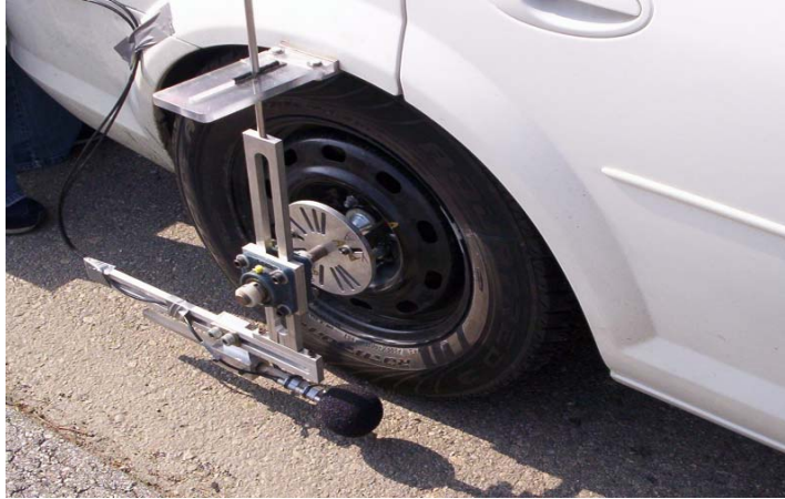
Figure 3: On-board sound intensity (OBSI) microphone setup.
